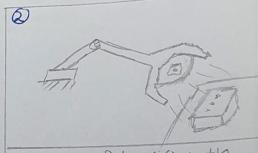
Correctly identifies the containers Id, snape size and colour using the autached sensors.
